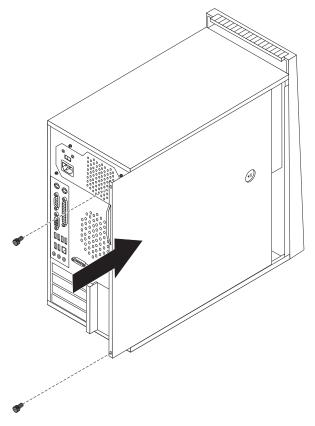
Figure 37. Reinstalling the computer cover
